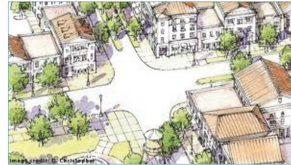
Figure 11.5 : Form-based code (FBC) illustration: FBCs use physical form, rather than separation of land uses, as their organizing principle.
